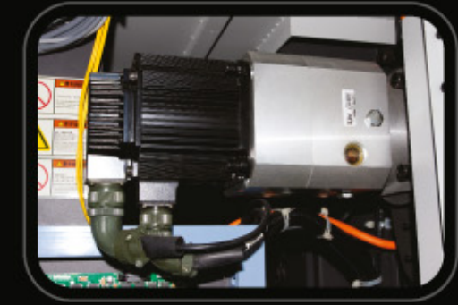
Servo Motor For Print Head Carriage and feeding System
